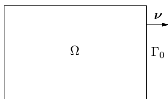
Figure 2.2. Outflow normal flux over a part \Gamma_0 of the outflow boundary \Gamma_+ of \Omega ; \boldsymbol{\nu} denotes the unit outward normal vector to \Gamma
